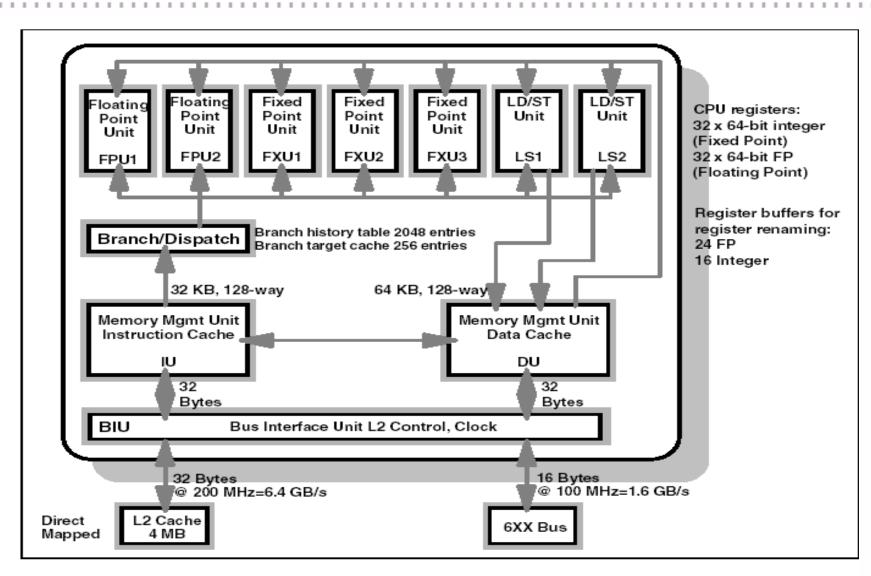
Figure 3. Model 170 - POWER3-II 400 MHz Block Diagram
