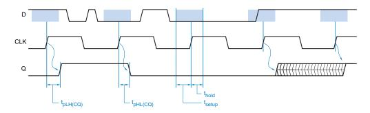
Figure 5: Timing Behaviour of a positive-edge flip-flop.
