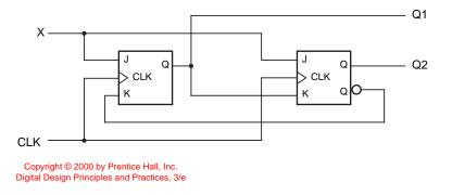
Figure 2: A sequential circuit using JK Flip-flops.
