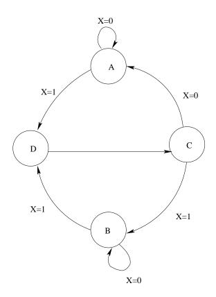
Figure 3: State Diagram for FSM implemented by circuit of Figure 2.
