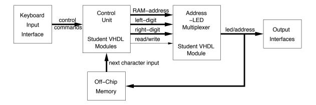
Figure 2: Block diagram for the Scrolling Message Display system.
