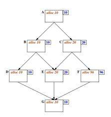
**Criterion 1:** For every control-flow path C of G, there will be enough registers allocated to allow the execution of every basic block of C.
