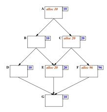
**Fig.5.** The *alloc* instruction are all necessary except the one in E for the control path [A, B, E, G].
