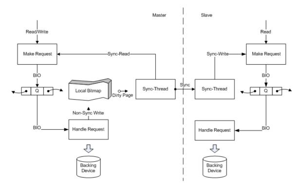
Figure 4.2: SBD Structure During Synchronization Stage
