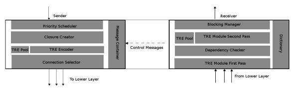
Figure 3.2: Architecture of the SMT layer
