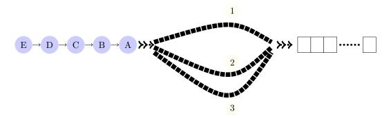
Figure 1.3: A stream of messages sent over a couple of connections.
