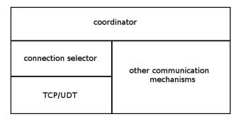
Figure 4.5: Architecture of the proprietary communication component
