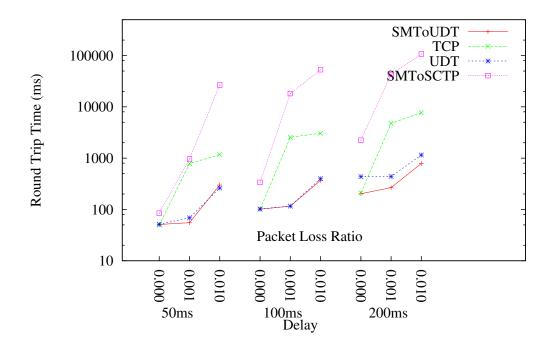
(b) RTT (lower is better); SCTP is missing because its average RTT is exactly the same as SMToSCTP.
