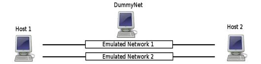
Figure 4.1: Test-bed used for running the benchmarks
