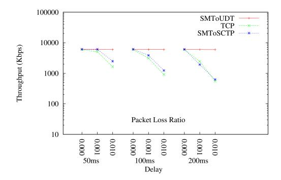
(a) Throughput (higher is better); UDT and SCTP are missing because their average throughput is exactly the same as SMToUDT and SMToSCTP respectively.
