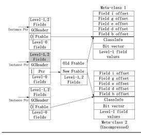
Figure 4. Field offset lookup mechanism
