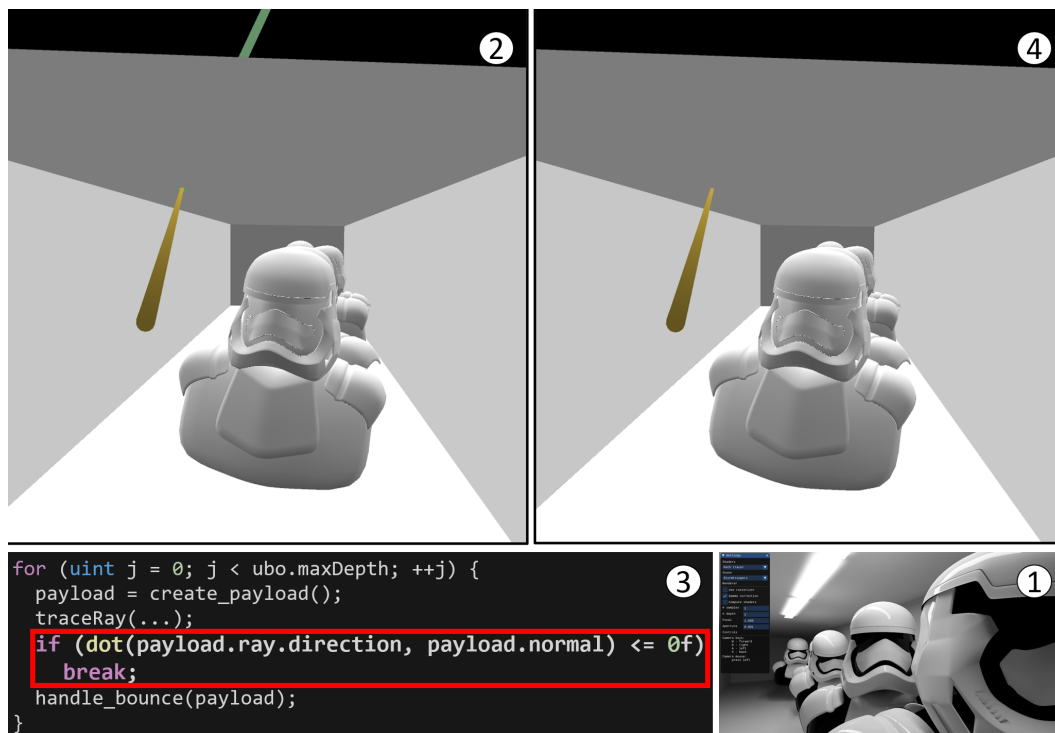
Figure 4.9: Top Left: RayScope’s visualization of PBRVulkan’s default path-tracing implementation. The yellow ray is generated from the camera. The green ray is the secondary ray incorrectly generated from the back-face of the box. Top Right: RayScope’s visualization of PBRVulkan after fixing a bug causing rays to be generated from the back faces of triangles. RayScope’s visualization shows that the green ray is no longer traced. Bottom Left: Pseudocode for our patch where our addition is outlined with a red box. The if statement terminates rays before they can be generated from the back faces of triangles. Bottom Right: Rendered image of PBRVulkan.
