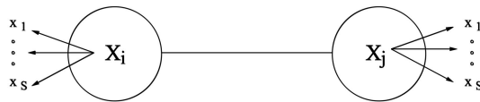
Fig. 2. Local “kernel” structure of the graphical model. Each random variable can assume S possible realizations, so that the sample space for two connected variables has S^2 elements.
