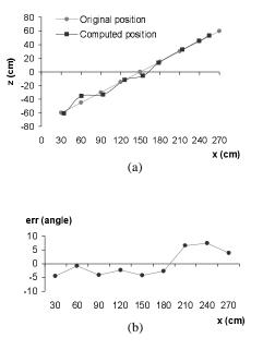
**Figure 7.** (a) Recovered positions from the 9 images. The first panoramic model is situated at (x, z)=(0, 0) and the second one at (x, z)=(300, 0); (b) Error for the recovered orientation. The x coordinates show the position of the planar image regarding the first panoramic model.
