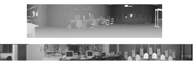
Figure 2: (top) Spherical representation of the range data from an  $180^{\circ}$  scan after filtering (bottom) Corresponding  $180^{\circ}$  panoramic mosaic.
