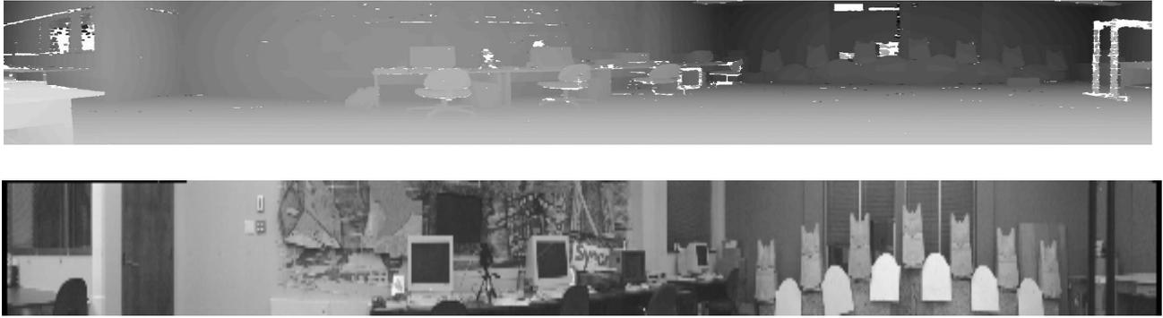
Figure 3: Spherical representation of the range data from an 180° scan after filtering (top). Corresponding 180° panoramic image mosaic (bottom).
