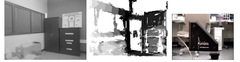
Figure 4.7: Example of a disparity map computed using the Triclops vision system. (a) left intensity image (b) disparity map (c) Triclops device
