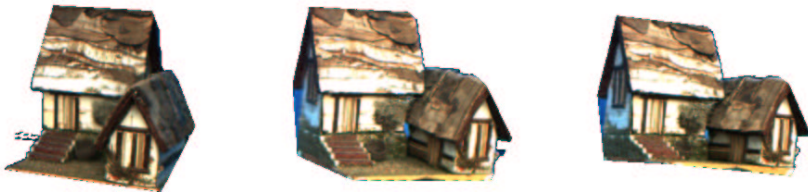
Figure 7.13: Rendered novel views of a house by modulating a texture onto a coarse captured geometric model. Note the absence of geometric distortions compared to the previous figure.
