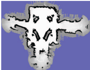
Figure 3.1: Example of occupancy map (white - free space, black - obstacle; blue - unexplored space) [152]
