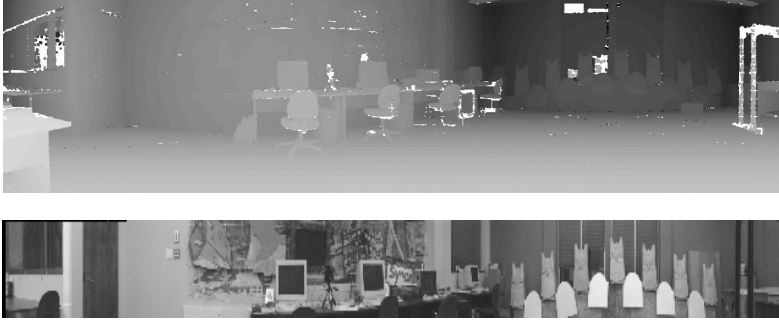
Figure 4.16: (top) Spherical representation of the range data from an 180° scan after filtering (bottom) Corresponding 180° panoramic mosaic.
