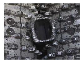
Fig. 6. Close-up of a shoveler's missing tooth stuck in the oilsand crusher. Image from Syncrude Inc.
