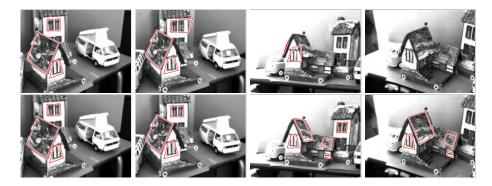
Fig. 2. Top Tracking individual patches using a homography. Not all regions can be tracked thought the whole sequence and occlusion is not handled. Bottom Through the 3D model each region motion is rigidly related to the model, and tracking succeeds through the whole sequence. The model also allows detection and removal of occluded regions and introduction of new regions. See supplied video1
