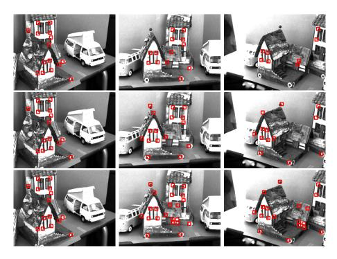
Fig. 3. Top Translation tracking of individual regions. Though the video sequence many patches are lost. Middle A projective 3D model is used to relate the regions, and provide more stable tracking through the whole sequence. Bottom An Euclidean model relates the region, and also allow the introduction of new regions. video2
