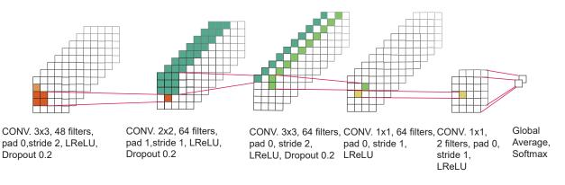
Fig. 2. State evaluation network architecture.
