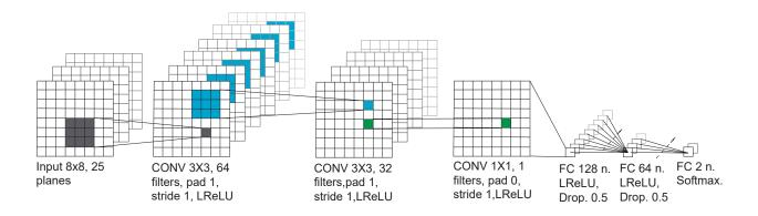
Fig. 1. Basic Convolutional Neural Network Architecture. Some layers aggregated (e.g.: CONV+LReLU).
