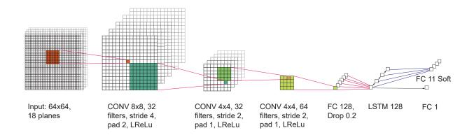
Fig. 5. Actor-Critic Network Architecture for TW battle scenarios, assuming maximum of E = 6 enemies (number of input planes = 12 + E, number of possible actions = 5 + E).
