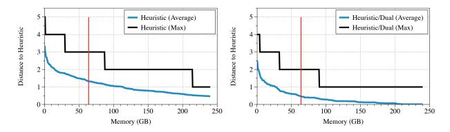
Figure 3: Measurements of the average and maximum distance to a heuristic lookup in the 12 edge PDB given that k GB have been loaded into RAM.
