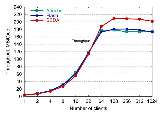
4-way Pentium III 500 MHz, Gigabit Ethernet, 2 GB RAM, Linux 2.2.14, IBM JDK 1.3
