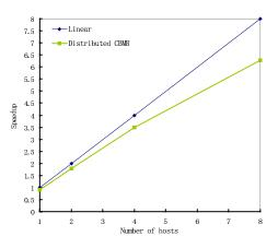
Figure 6. Speedup of distributed CBIR application. Image database size: 600MB
