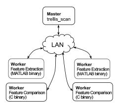
Figure 4. Control flow of CBIR application
