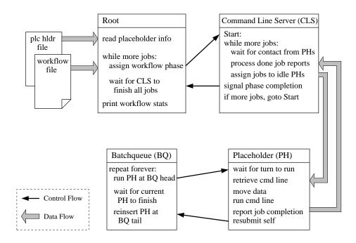
Figure 6.1: Control and Data Flow in Smurph Simulator
