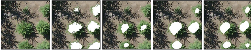
Figure 4. Longer operator sequences lead to better labeling. From left to right: the original image, desired user-provided labeling, the best labelings with an operator sequence of length 4, 5, and 6.
