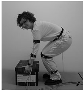
Fig. 3. Lifting a heavy object. The movement sensors were placed on the hip, above the knee, above the foot, on the upper arm, on the forearm, and on the hand of the left body side.
